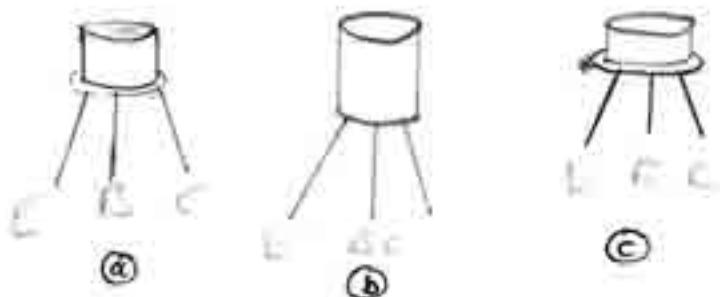
Fig(5): Transistor package types
